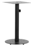
CIRCLE TABLE DINING BASE 4301+FINISH 94,97 W19.75" D19.75" H29" Use tops: 24"-36" Hole spacing: 24"
